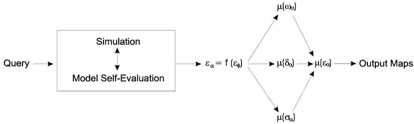
Fig. 3. Flow of processes within the decision support system. RHESysD is contained within the box, while all components to the right of the box are considered part of the decision support system.
