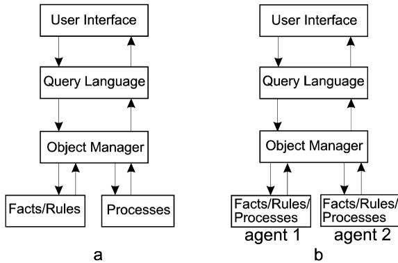
Fig. 1. Model-based management can be approached from the perspective of the model as (a) black-box, or (b) an integral part of the software system in which all components, e.g., sub-models, must be viewed as acting together towards achieving a common goal.
