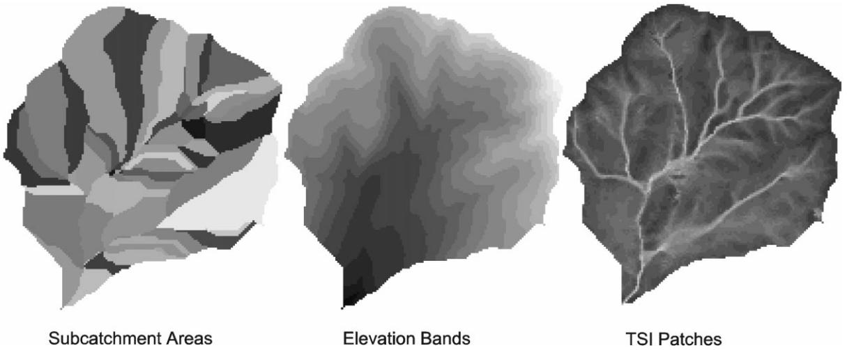
Fig. 6. Partitioning of Onion Creek into subcatchment areas, elevation bands or zones, and TSI patches for spatial representation of input to RHESSysD.
