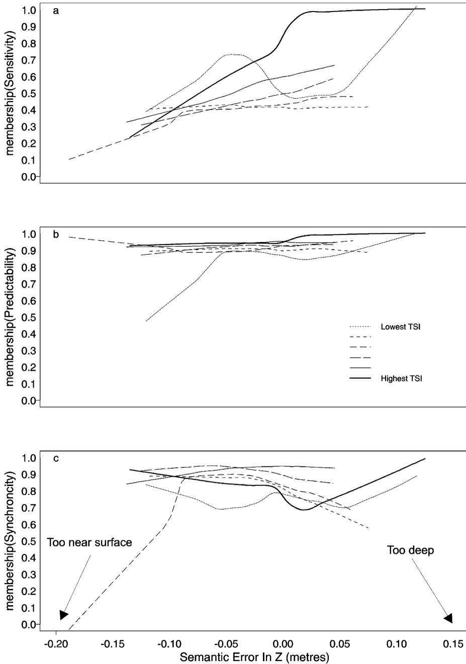
Fig. 8. Plots of (a) sensitivity memberships, (b) predictability memberships, and (c) synchronicity memberships for soil moisture versus semantic error in the water table, for each of the respective aggregate TSI zones.
