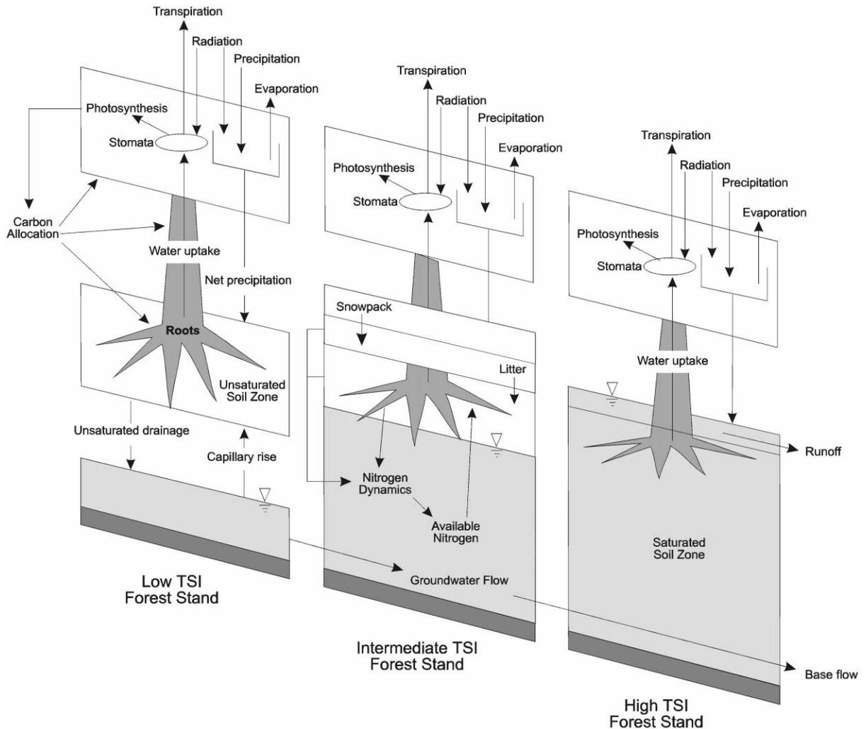
Fig. 4. Physical processes represented by RHESSysD. Shown are three patches (e.g., forest stands) with vertical water fluxes and horizontal water fluxes.
